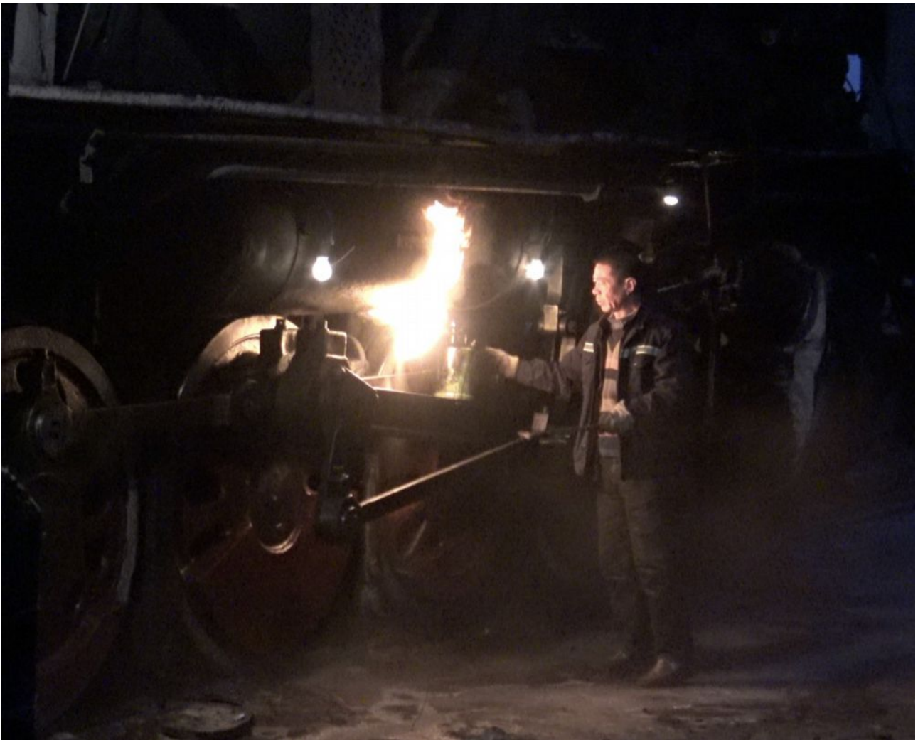
The water drain cock for the air reservoir needed unfreezing before eventually the Westinghouse pumps kick into action.
