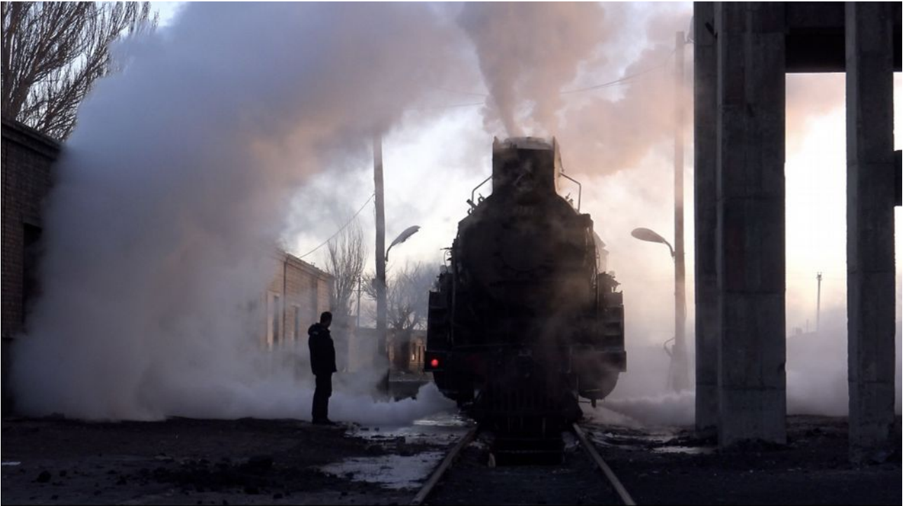
Steam is released from the cylinder drain cocks to warm up the cylinders and clear any ice and water.
