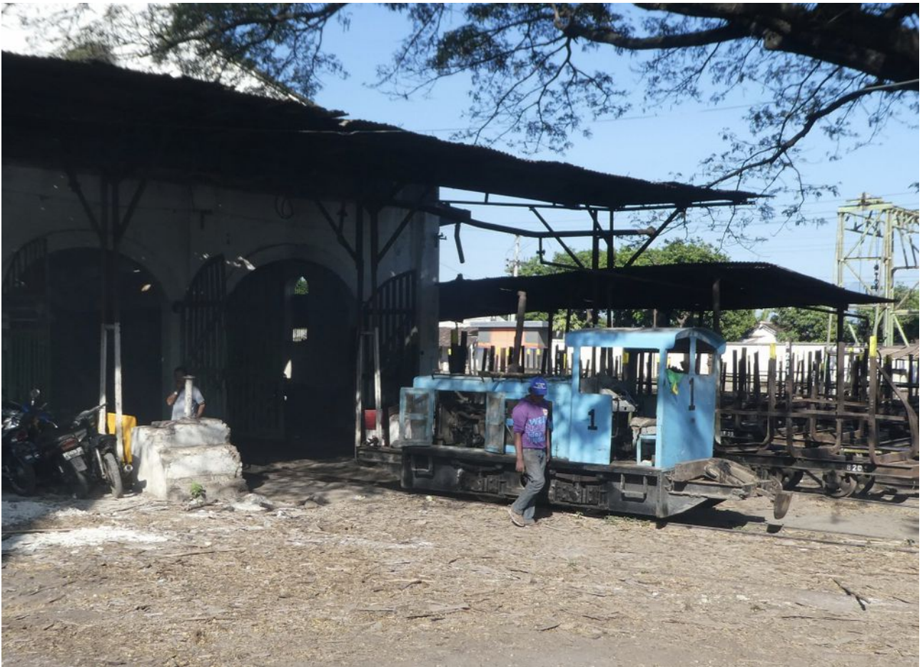
Kyosan Kogyo No. 1 is still working but produced clouds of smoke from all parts of the engine rather than the exhaust pipe. It clearly has a smaller (non-original) engine to KK No. 2.
