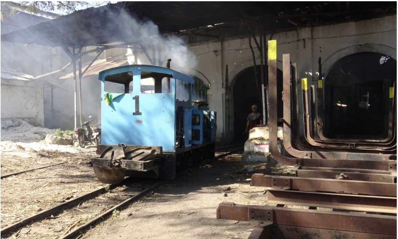
Kyosan Kogyo No. 1 is still working but produced clouds of smoke from all parts of the engine rather than the exhaust pipe. It clearly has a smaller (non-original) engine to KK No. 2.
