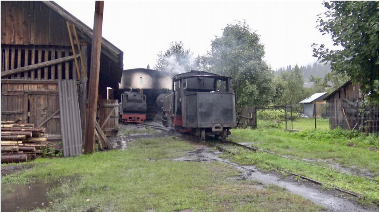
There is a stubby tender once hauled behind the locos but now used only for coaling the loco rear coal bunker.
